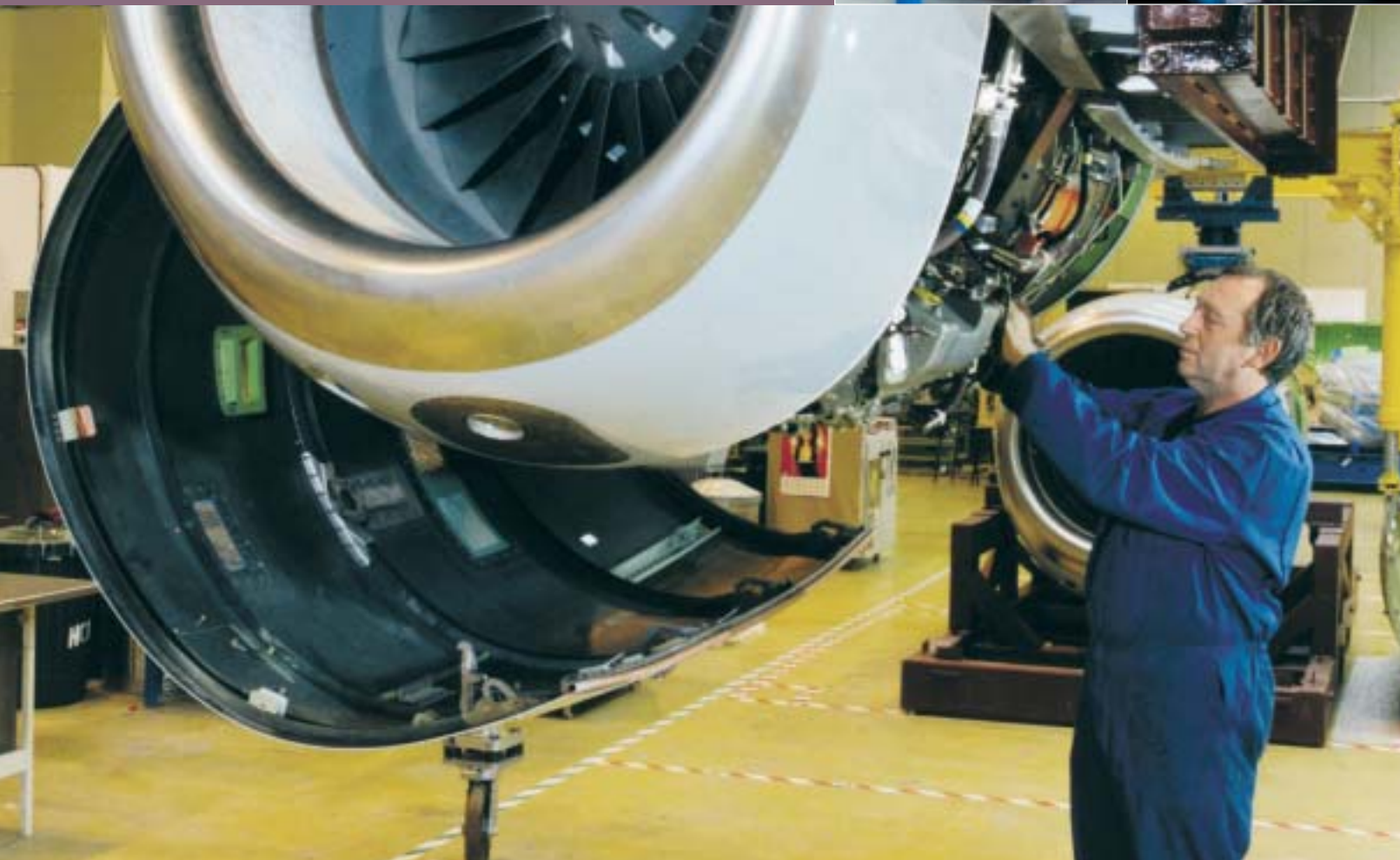
BELOW Assembly of AS907 nacelle used on the Bombardier Challenger 300
