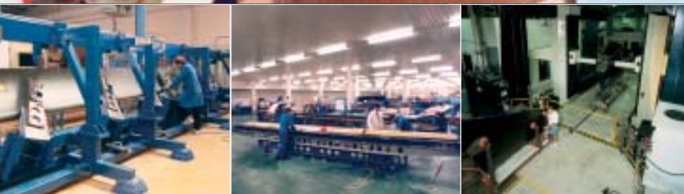
ABOVE Lay up of an F-18 horizontal stabiliser LEFT C-17 flap vane assembly CENTRE Composite clean area RIGHT Automated ultrasonic scanning system
