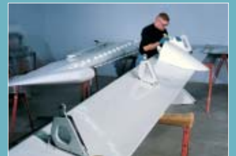
Repair of composite wing component
