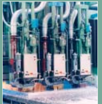
Droop and Rein 3-axis CNC long bed milling machine
