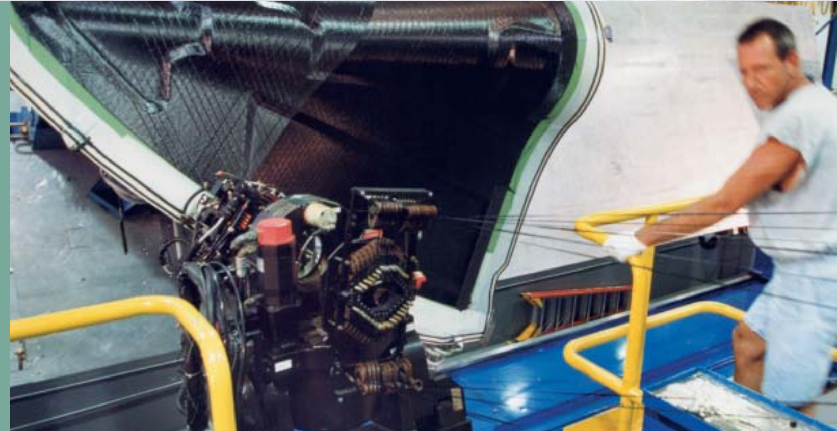
ABOVE Ingersol 7-axis CNC Fibre placement machine LEFT Filament winding of a Black Hawk refuelling probe CENTRE A340 500/600 overwing panels RIGHT Automated trim and drill BELOW Lay up of a Trent 500 fan cowl door
