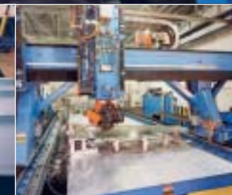
ABOVE Ingersol 7-axis CNC Fibre placement machine LEFT Filament winding of a Black Hawk refuelling probe CENTRE A340 500/600 overwing panels RIGHT Automated trim and drill BELOW Lay up of a Trent 500 fan cowl door
