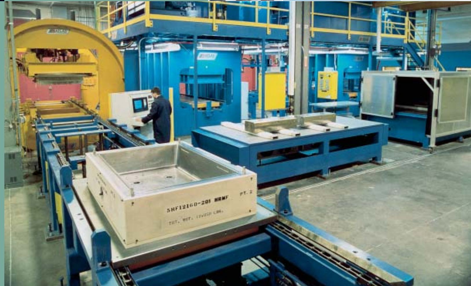
LEFT Sine wave wing spar CENTRE Engine thrust reverser cascade RIGHT Helicopter main rotor hub BELOW Computer controlled flexible resin transfer moulding machine
