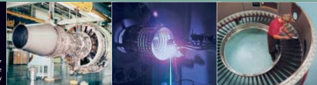
LEFT Acoustic nozzle for Boeing 757 MIDDLE Coating of a high pressure compressor case RIGHT Trent Fan Case Assembly
