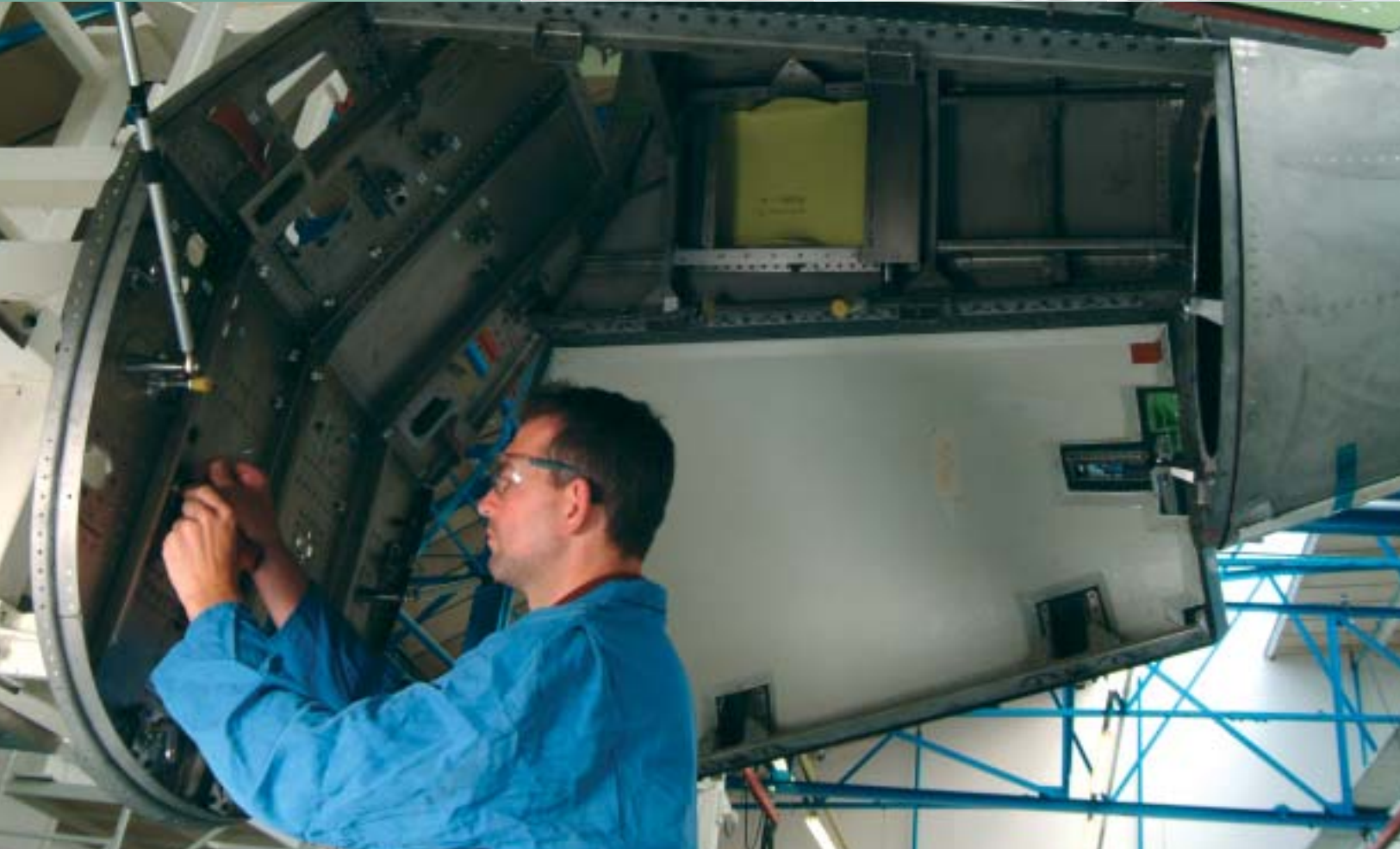
LEFT F/A-22 welded titanium boom CENTRE A340 Shroud box RIGHT A340 500/600 aft pylon fairing BELOW Assembly of Bombardier CRJ700 tailcone
